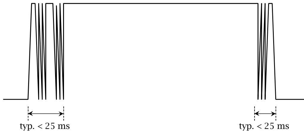
Figure 10: Typical Switch Contact Bounce
